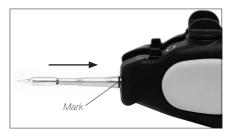
Insert the cartridges as far as the mark for a proper connection. Before inserting, make sure the cartridges are clean to ensure the proper functioning of the tool.
