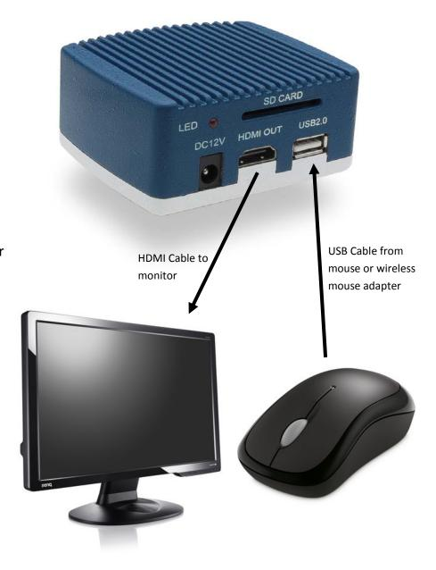
When using camera in HDMI mode you can connect the provided mouse to the camera via the USB port on the back of the camera. Move the mouse cursor to the bottom of the screen to make the HDMI Mode control bar appear. When you move the mouse away from the control bar it will disappear.
