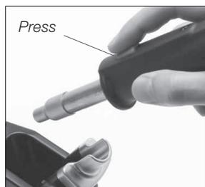
Press the start/stop button to blow hot air.
