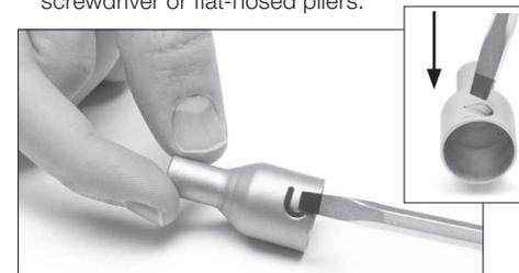
2. Insert the nozzle into the JT-TA Heater again.
