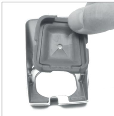
6. Insert the new one and reassemble
