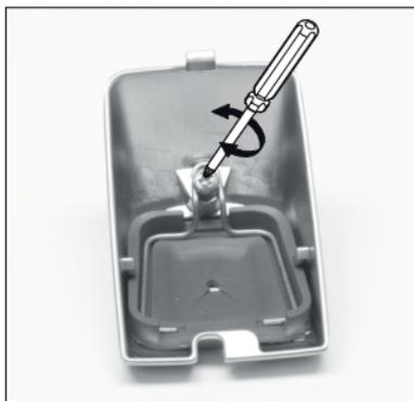
4. Remove the retainer spring
