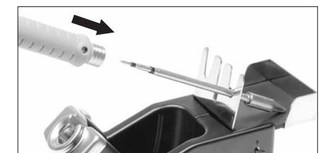
Insert the new cartridge and press slightly as far as the mark\* and tighten the screw.
