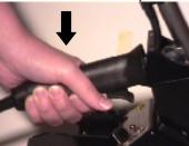
While Tool is in the Pod, push handle down and twist handle until it locks into 1 of it's 4 positions. Twisting counter-clockwise will permit a 180° turn. Twisting clockwise will permit a 90° turn.
