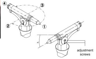
To tilt the Head assembly, loosen (2) Adjustment Screws. Tilt the Head assembly to desired position. Retighten Screws.
