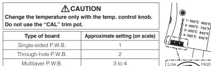
• In general, the greater the temperature, the more quickly the nozzle will oxidize and wear out.
