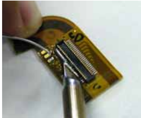
2. For flow soldering or modifying solder bridges
