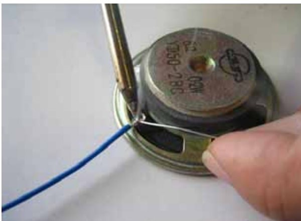
5. For lead wire soldered to the terminal pin of speaker, connector, switch etc
