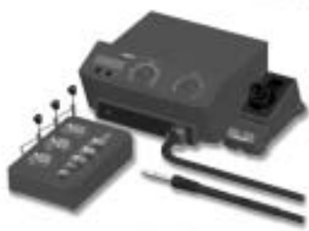
TE 5000 Precision hot-air station
